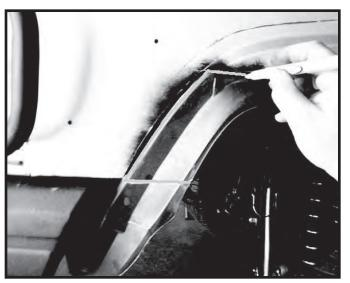
Step 18. Fold the wheel well liner flap forward near the front bumper. Draw a line on the inside of the liner from the corner of the fender by the marker light diagonally down to the outside of the first mounting hole. Trim on the line that was created. It may be necessary to secure the front area of the liner to the inside of the wheel well.
