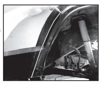
Step 11. Draw a horizontal line from the contour line inward towards the wheel well at the top of the third bolt hole. Repeat for opposite side.
