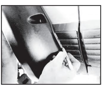
Step 21. Using a putty knife lift the body trim off of the body enough to cut with a razor knife.
