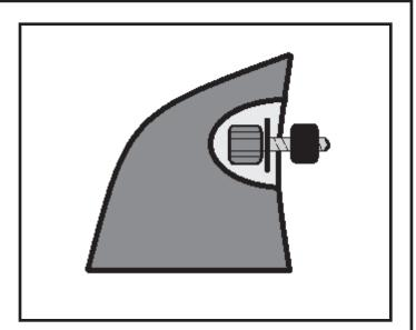
Step 27. Place the flare against the body and align the screws into the drilled holes in the body. Tighten the screws. Do not torque over 24 inch pounds.
