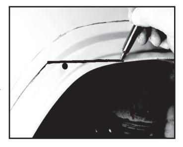
Step 9. Mark a line 5 1/4" from the edge of the fender at the front door jam towards the fender well at the bottom of the vehicle.
