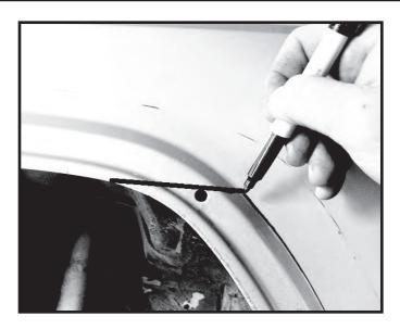
Step 12. Begin trimming the marked areas. Use of an air saw or grinder will be needed. You must wear eye and ear protection when cutting metal. Gloves should be worn when handling sharp metal. Use caution when cutting metal. Do not over cut. Ensure the are no obstructions on the back side of the metal being cut.
