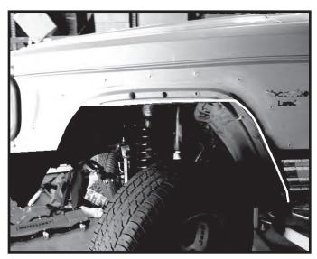
Step 15. Trim the inner seam at the rear of each front fender well. The inner seam should match the outer cut fender. The cut piece from the outer fender can be used as a template. A sanding wheel should be used to even out the cut areas.
