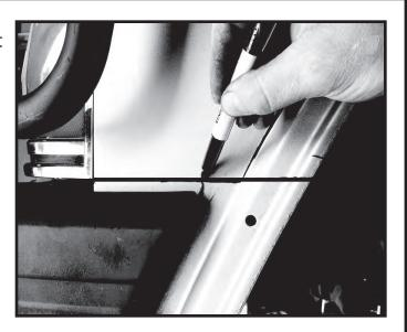
Step 6. Using the line previously drawn measure 5 Inches in towards the wheel well starting from the headlight bezel and place a mark. Repeat for opposite side.
