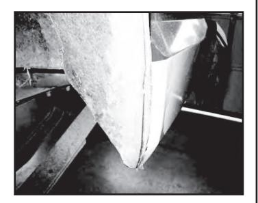
Step 36. Cut area # 5 in steps. Trace a line following the contour of the raised flare out of the body. Trim only the outer skin in the area outlined. The remaining area should be cut through both layers and removed. Repeat for opposite side.
