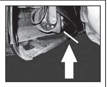
Step 14. When cutting is finished the front fenders should look like the image. All edges should be smoothed and free of burrs. All exposed metal must be treated before flares are installed.
