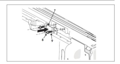
6. Prior to placing the cover, remove both front clamp knobs.
