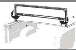
Open the tailgate, swing the tail clamps down from the stowed position and silde them toward the truck bed rail. Swing the clamps and pull down so the clamp jaw is tucked under the rear truck bed rail bracket.
