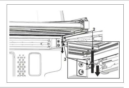
8. Thread the cab clamp knobs back onto the threaded rods.
