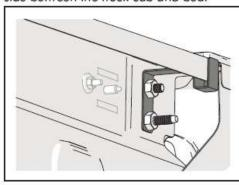
Rear/tailgate Brackets. Attach the rear/ tailagte brackets (7) to the bed rail through the bed rail holes using the rear bracket bolts (8).
