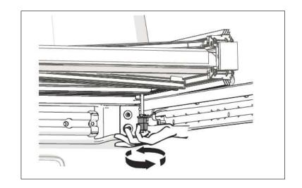
Close the tailgate and unfold the cover. Check that the cover is parallel and square with the truck bed and bed rails.
