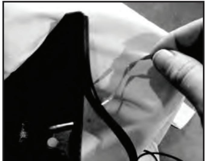
Step 25. Clean inside mounting lip edge with rubbing alcohol. Install edge trim as shown by removing red vinyl tape covering only a few inches at a time. Do not stretch the trim while being applied, this may cause shrinkage after installation.
