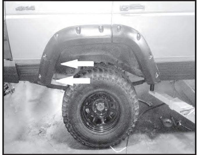
Step 41. Use of the trim tool may need to be used on any parts of the trim that have been misaligned during installation. To seat the trim against the body, the curved side will be used. To seat the trim side against the flare the flat side will be used. It may be necessary to start at one end and run the tool the full length of the flare.
