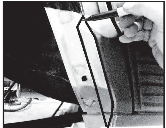
Step 37. Fold the metal flap created to close the gap between the inner and outer sheet metal. All edges should be smoothed and free of burrs. All exposed metal must be treated before flares are installed. A filler putty may be used to seal the area. Repeat for opposite side.
