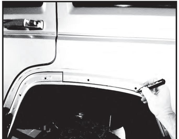
Step 34. Cut out the rear fender in the order shown. Starting with #1 area trim the 3/8 inch lip from the fender. Area's # 2, 3 only trim down to the body moulding area. Area # 5 only cut the outer skin in this area. See next steps for areas # 4, 5. Repeat for opposite side.
