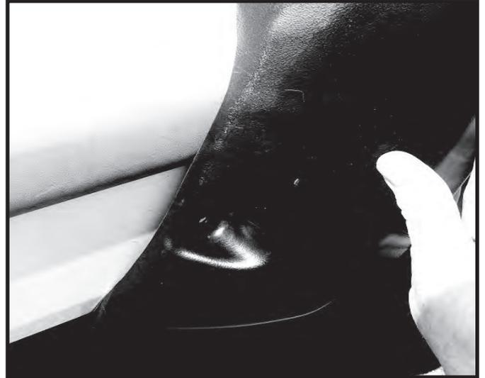
Step 23. Drill the mounting holes using a 3/16" drill bit.
