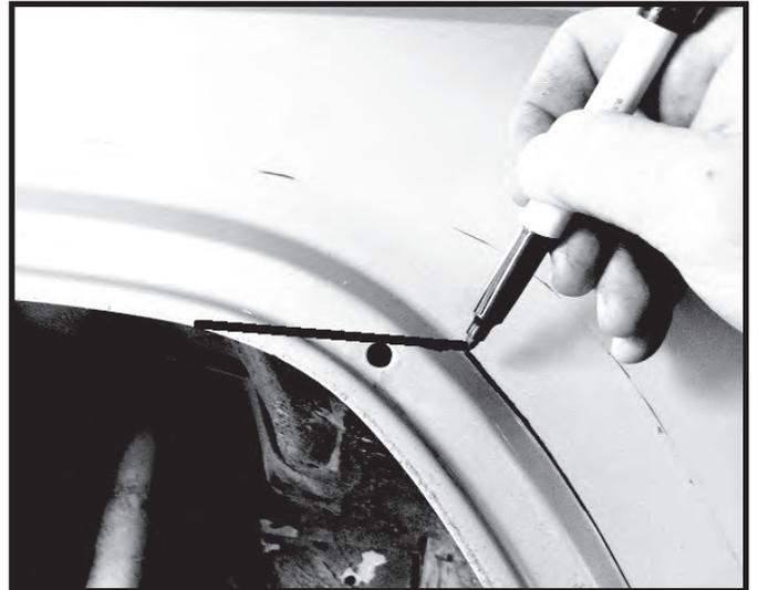
Step 12. Begin trimming the marked areas. Use of an air saw or grinder will be needed. You must wear eye and ear protection when cutting metal. Gloves should be worn when handling sharp metal. Use caution when cutting metal. Do not over cut. Ensure there are no obstructions on the back side of the metal being cut.
