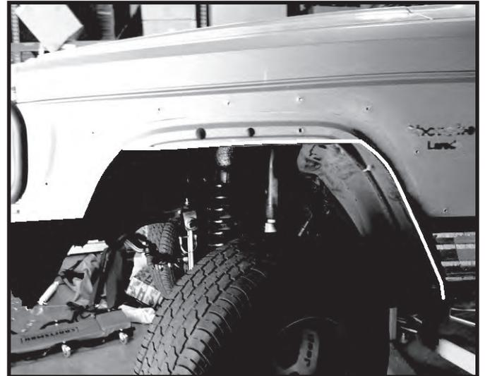
Step 15. Trim the inner seam at the rear of each front fender well. The inner seam should match the outer cut fender. The cut piece from the outer fender can be used as a template. A sanding wheel should be used to even out the cut areas.
