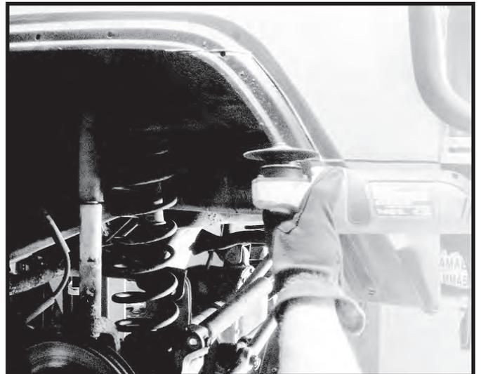
Step 13. Cut the lower fender brace close to the frame. Repeat for both sides.
