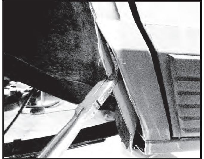
Step 38. Install the dog leg shaped trim piece on the door edge. At the rear door opening fit the trim against the body. Secure the trim in place with the supplied self tapping screws. Use the dimples in the plastic as guides for the screws. Do not overtighten. Repeat for opposite side.
