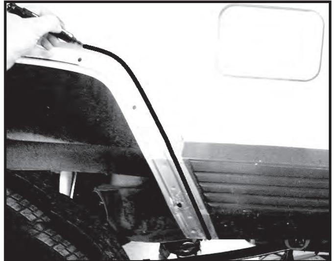
Step 33. Measure 3/8 inch up from the edge of the fender well and draw a horizontal line along the fender connecting the two lines made in the previous steps. Repeat for opposite side.
