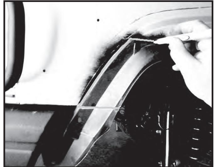
Step 18. Fold the wheel well liner flap forward near the front bumper. Draw a line on the inside of the liner from the corner of the fender by the marker light diagonally down to the outside of the first mounting hole. Trim on the line that was created. It may be necessary to secure the front area of the liner to the inside of the wheel well.
