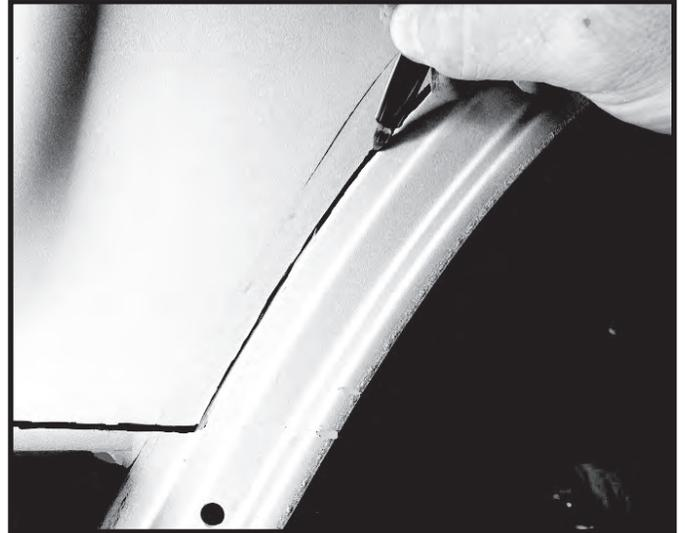
Step 8. Trace a horizontal line from the previous line in step 7 toward the inside of the fender well at the top of the third factory mounting hole. Repeat for opposite side.
