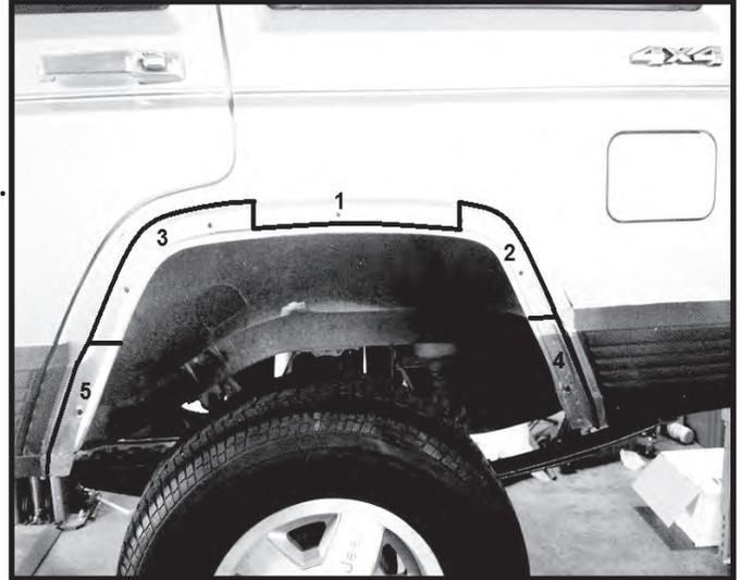
Step 35. Cut area # 4 carefully. Start by cutting 3/8 inch from the line and grind the rest of the way. A filler putty or silicone is needed to fill the gap between the sheet metal. Repeat for opposite side.
