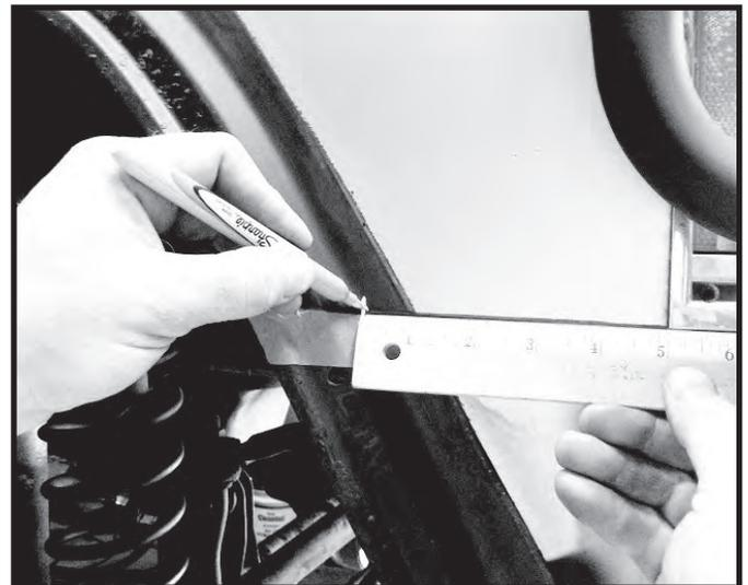
Step 7. Following the contour of the raised area on the fender, trace a line upwards to the top of the third factory mounting hole. Repeat for opposite side.
