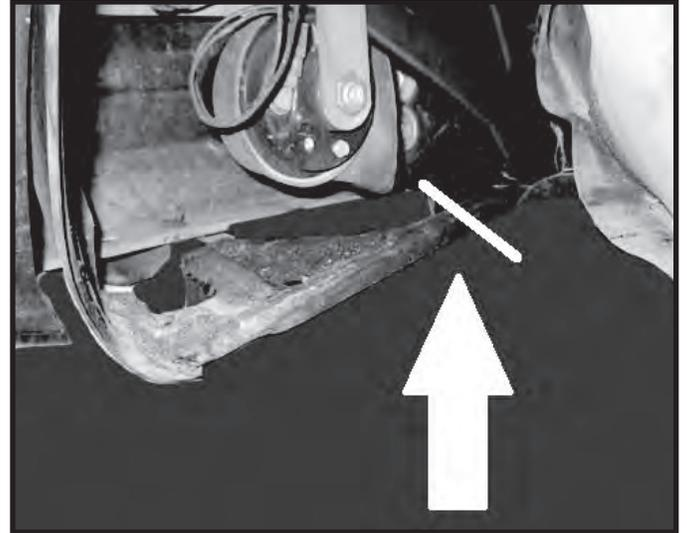
Step 14. When cutting is finished the front fenders should look like the image. All edges should be smoothed and free of burrs. All exposed metal must be treated before flares are installed.
