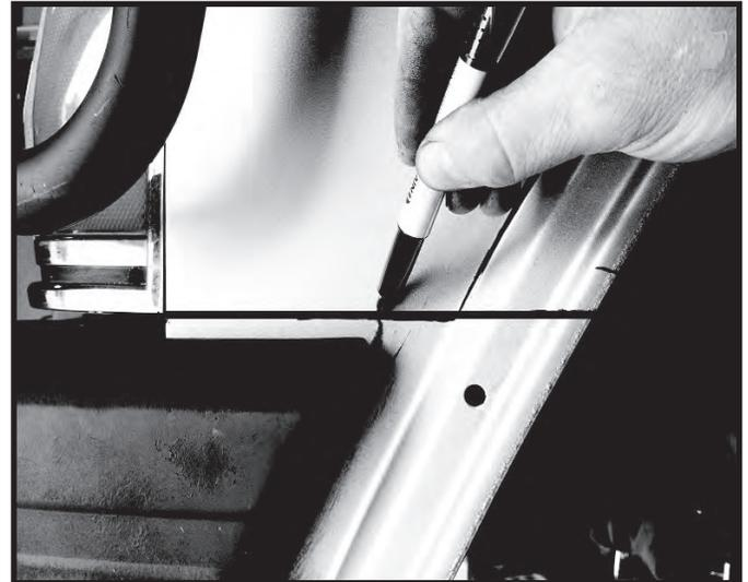
Step 6. Using the line previously drawn measure 5 Inches in towards the wheel well starting from the headlight bezel and place a mark. Repeat for opposite side.
