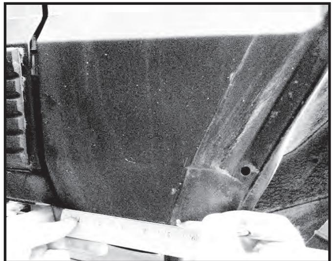
Step 10. Starting at the mark made in the previous step draw a line upward following the contour of the raised area on the fender to the top of the third factory bolt hole. Repeat for opposite side.
