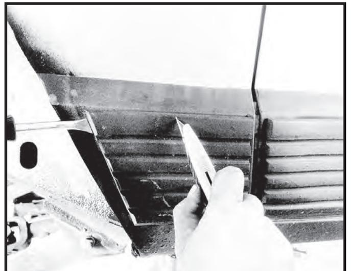
Step 22. Once fitment is complete hold the flares in place and mark the mounting holes on the body using the pre-drilled holes in the flare as a guide.
