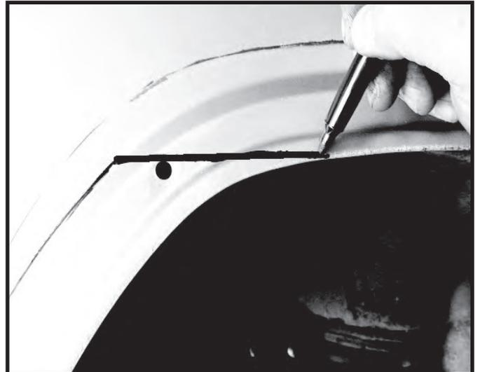
Step 9. Mark a line 5 1/4" from the edge of the fender at the front door jam towards the fender well at the bottom of the vehicle. Repeat for opposite side.
